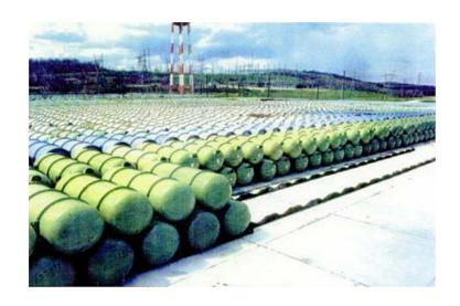
Depleted U<sub>3</sub>O<sub>8</sub> from the gaseous diffusion plants (GDPs) is packaged in diffusion plant cylinders
